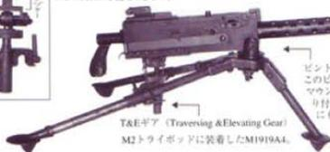
T&Eギア (Traversing & Elevating Gear)
